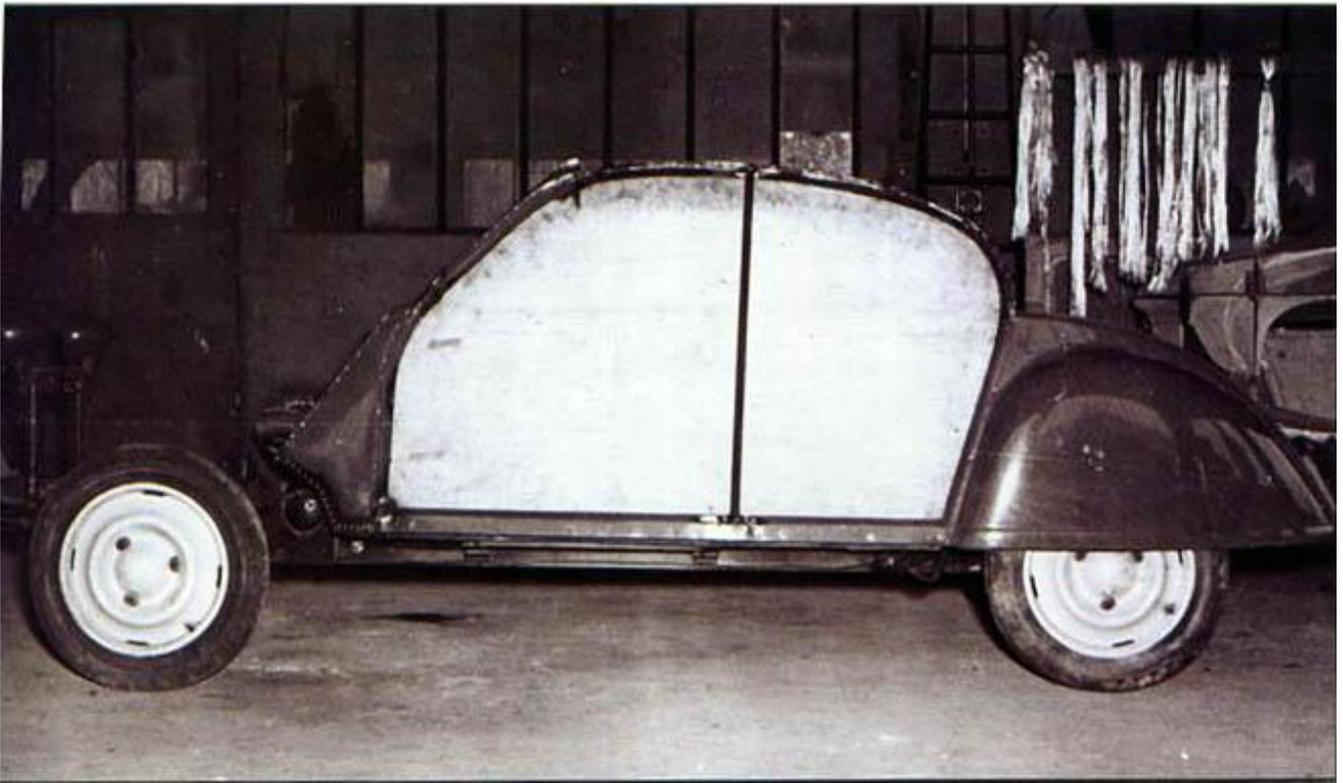
*The body of the 2 CVA was removed and another body, with better rear fenders, was put on the frame. Once the panel beaters had finished, 18 centimetres were reduced. The top of the car now marries perfectly with the template and the centre post has been moved back. The height of the dashboard was brought down from 67 to 57 centimetres by decreasing the aforementioned in the lower half.*
